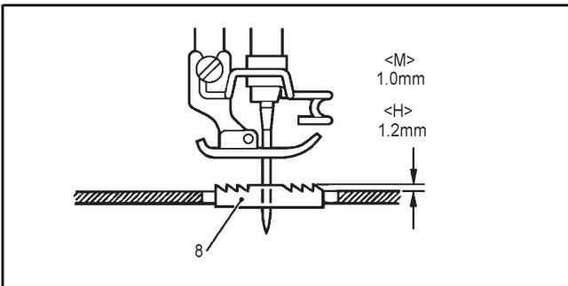
1. Turn the pulley until the feed dog (1) rises to the highest position.
