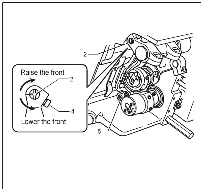
If you would like to tilt the feed dog (1) further. turn the feed lifting rock bracket stud (5) while carrying out the above adjustment (Fig [D])
